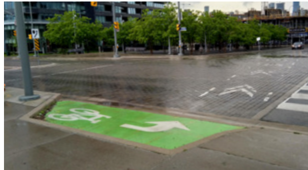
Figure 6.52 – Example of a Pocket at T-Intersection, Toronto
