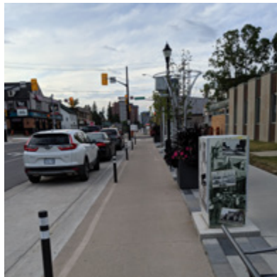
Cycle Track Separated by Mountable Curb and Parking Lane, Waterloo
