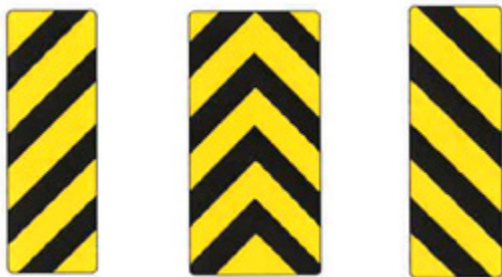
Wa-33R (OTM) (300 x 900 mm) Wa-33LR (OTM) (450 x 900 mm) Wa-33L (OTM) (300 x 900 mm)
