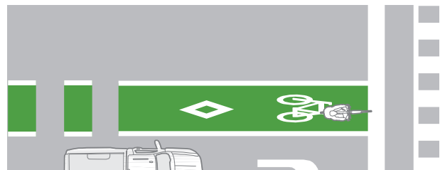
Figure 6.12 – Solid Green Treatment on Intersection Approach
