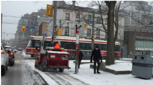
Figure 10.22 – Sidewalk Plow Clearing Cycle Track, Toronto
