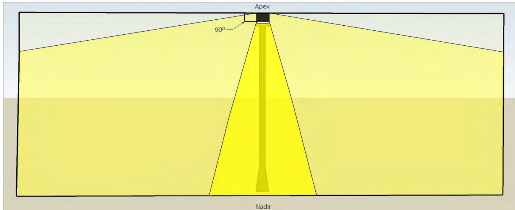
Figure 3: Full Cut-off Fixture
