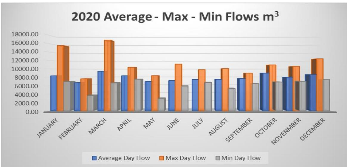
Figure 3: Monthly Average, Max and Min Day Flows in m³ for 2020.
