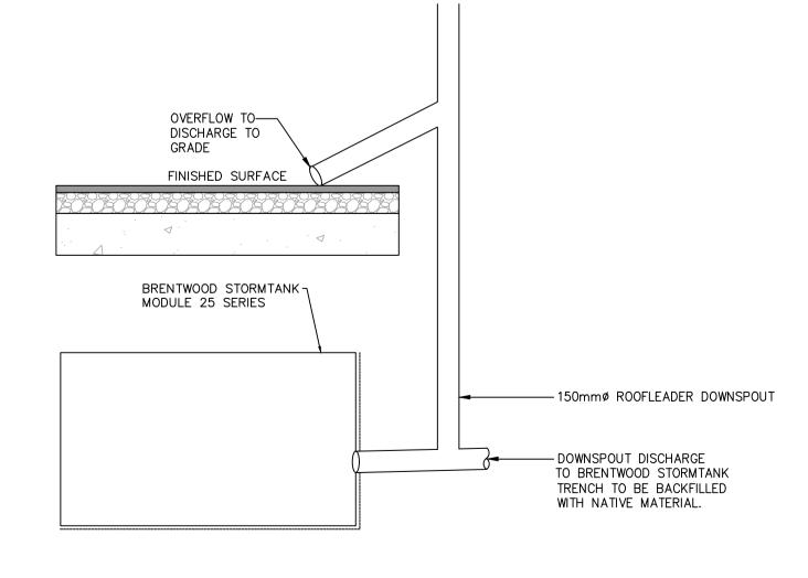
ROOF DOWNSPOUT DETAIL
